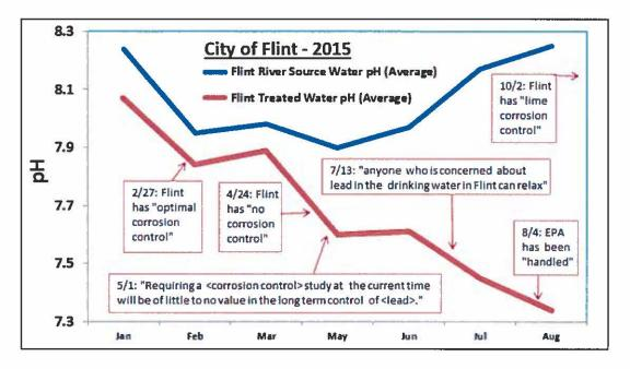
of 2015 and that it increased after June. By comparison, the graph shows that the pH in Flint's municipal water supply started dropping steadily from 7.9 S.U. in March (just after Veolia made its recommendation to double the ferric chloride concentration) to 7.3 S.U. in August. This difference is significant because pH is measured on a logarithmic scale, which means that a pH
